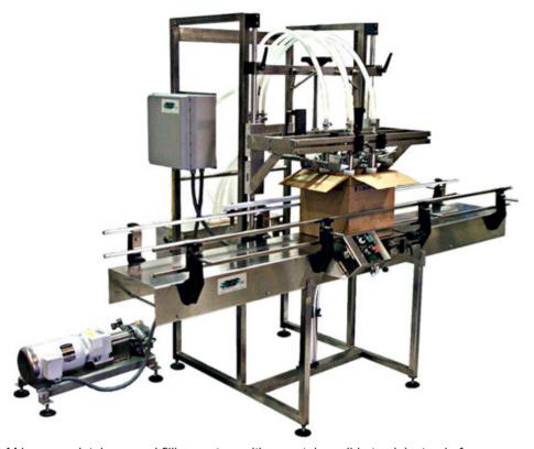
The ILS-M is a completely manual filling system with a container slide track instead of a power conveyor. The containers must be pushed in and out of the fill zone manually. The operator controls the movement of the nozzle spout bar and operation of the pump via manual switches and levers. The system is used for low volume, pilot runs, or situations which do not justify a fully automated system.
