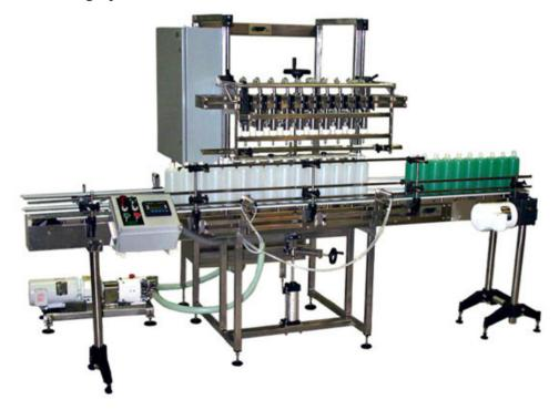
A fully automated system supplied with a 10 foot, powered conveyor with programmable logic controller (PLC) and container sensors control the machine functions.
